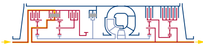
3 rd Gear At approximately 50 % (or 70 % with D 851.3E/D 863.3E) of the maximum speed, the input clutch opens automatically and the 3rd gear clutch is closing.
