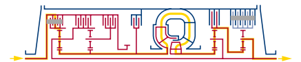
Reversing (R) Power is transmitted hydrodynamically/ mechanically as in 1 st gear (DIWA driving range).
