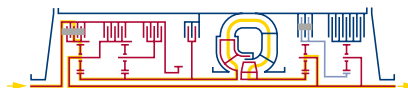
1 st Gear DIWA range (stepless), input clutch and turbine brake are closing: smooth start with high traction. Rapidly increasing mechanical power transmission via differential transmission (power-split principle).
