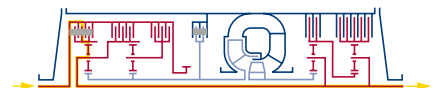
2 nd Gear Automatic gear shifting is dependent on acceleration and driving speed: Impeller closes, turbine brake opens. Power is now transmitted purely mechanically.
