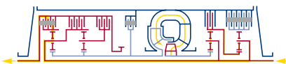
Braking (in 2 nd – 4 th gear) (Retarder function with the converter) The turbine wheel acts as axial pump which delivers oil against the stalled impeller and the guide wheel. Heat resulting from the conversion of kinetic energy is dissipated via the heat exchanger.
