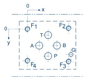
View: fastening side of mounting plate F: M5, thread depth min.  $1.5 \times \emptyset$  G: bore hole depth min.  $1.5 \times \emptyset$
