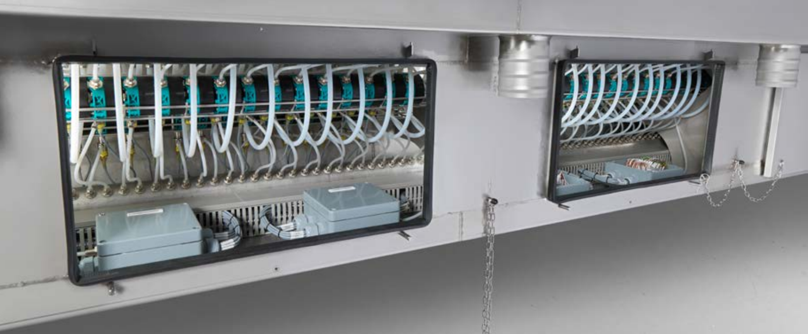
OnQ ModulePro DG maintenance ports and integrated valves
