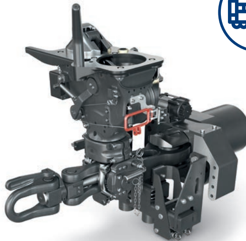
Coupler head swiveled upwards: ready for connection with drawhook
