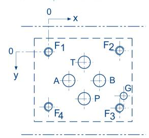
View: fastening side of mounting plate F: M5, thread depth min. 1.5 x  $\varnothing$  G: bore hole depth min. 1.5 x  $\varnothing$
