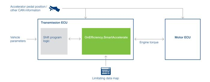
OnEfficiency. SmartAccelerate limits the engine torque emitted via CAN, in order not to exceed a given vehicle acceleration. To achieve this, OnEfficiency. SmartAccelerate defines for each DIWA shift program a specific data map with the acceleration limit in relation to the vehicle speed range.
