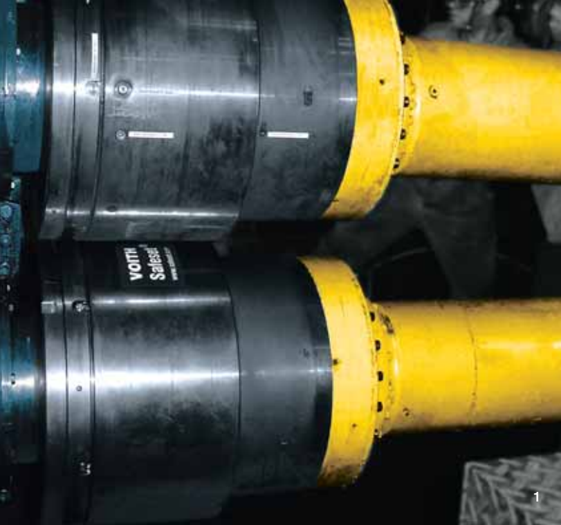
1 SR-F 560 Integrated with gear spindles in a stripmill
