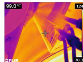
Cast iron cylinder with uneven temperature at shell edge
