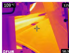
Steel cylinder with even surface temperature
