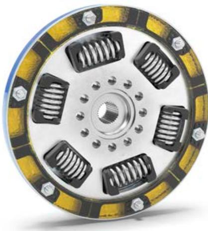
During low torsional vibration, the HP Coupling operates in the isolation range where the damping ring absorbs and isolates vibrations within the defined backlash range (Fig. 2). This keeps the power loss of the test rig at a minimum and allows very precise test results. The viscous-hydraulic damping and the isolation function give the coupling optimal damping behavior across the entire nominal speed range.
