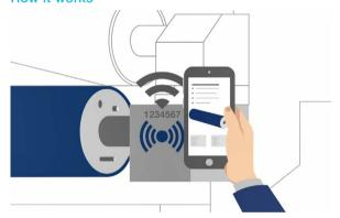
The module "ID Tagging" is a combination of wireless connectivity technologies and the integration of digital nameplates. The solution offers a simple and user-friendly identification of rolls and fabrics, through a simple scan of a tag.
