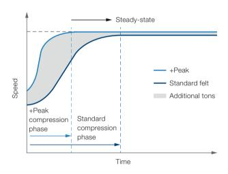
A standard press fabric must overcome a break-in period before the paper machine can reach its expected operation levels. The felt will become saturated during a compression phase to reach an optimum dewatering at maximum speed. As +Peak enables a higher saturation capability during startup, the felt will reach the optimum efficiency in a much shorter time. Therefore, a faster startup results directly in a higher production.
