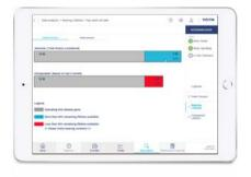
Operating torques can be analyzed retrospectively and provide information about potential for equipment optimization. The maximum torque occurrences are archived in high resolution, which allows an accurate analysis and at the same time ensures that the drive is operated within the component specifications.
