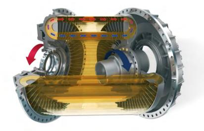
The coupling operates on a constant quantity of operating fluid, usually mineral oil. On demand, design for water is available. The torque transmitted by the drive motor is converted into kinetic energy of the operating fluid in the pump wheel to which the motor is connected. In the turbine wheel, this kinetic energy is converted back into mechanical energy. Three operating modes are defined:
