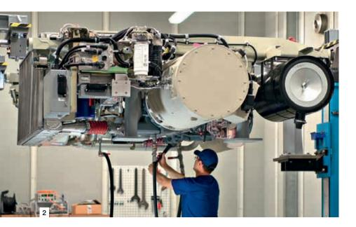
class resulting in improved driving comfort due to minimum vibration and low noise levels. Voith RailPacks also meet the most strict emission standards for rail vehicles. They can help reduce fuel consumption up to 8% while delivering 23% more power than comparable drive systems using the same installation space.
