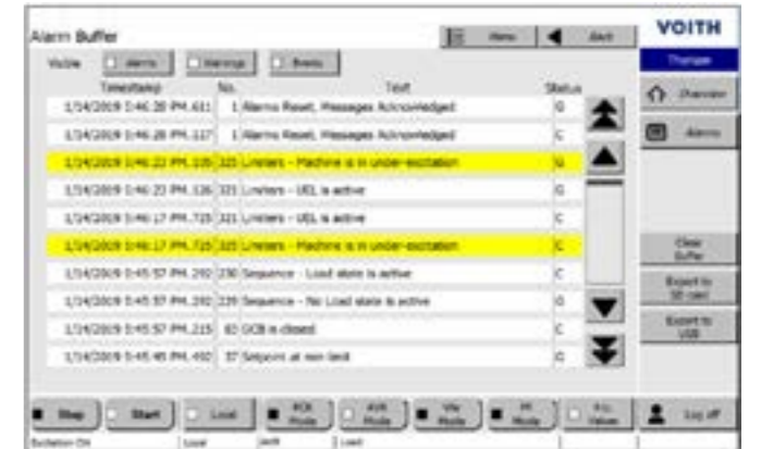
Alarms and events buffer screen are exportable as text files to USB or SD card directly from the operator panel
