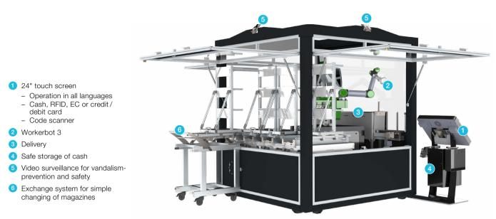
The Workerbotkiosk is a fully automated shop in the format of a kiosk. Nobody works in the store, but just a robot.
