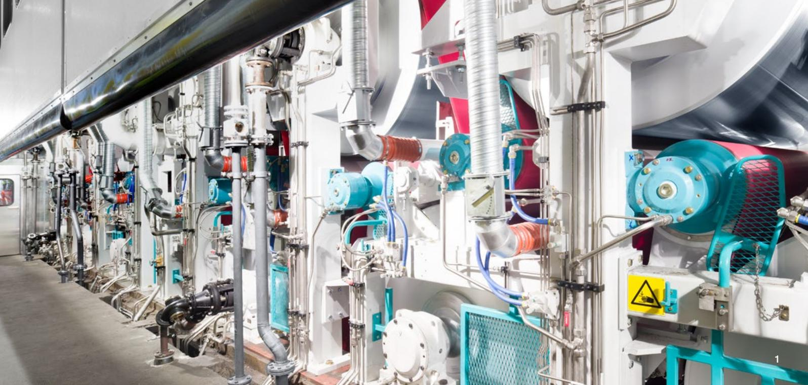
All over the world, paper manufacturers are facing the challenge of ensuring consistently high or superior paper quality while at the same time reducing their investment and production costs. With EvoDry steel cylinders, Voith is revolutionizing the paper drying process and facilitating improved papermaking at the highest level of efficiency.
