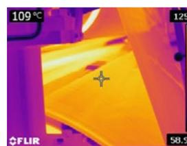
Steel cylinder with even surface temperature
