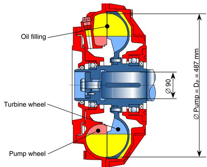
Fig. 2: Cross section of VTC 487 T coupling
