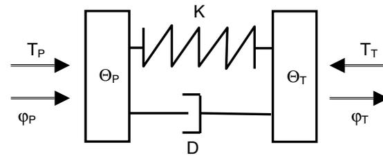
Fig 1: Kelvin Model (Indices: P = Pump; T = Turbine)
