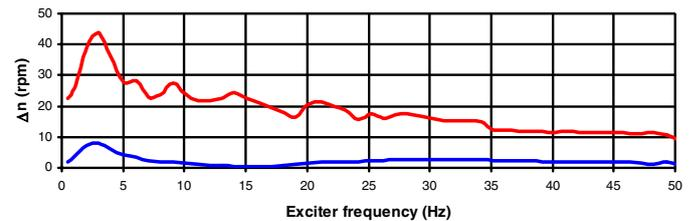
Fig. 8: Measuring values – speed amplitudes of pump side (red) and turbine side (blue)
