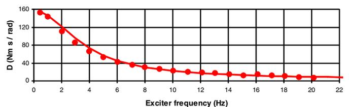
Fig. 10: Damping D – Measurements (dots); Theory (continued)
