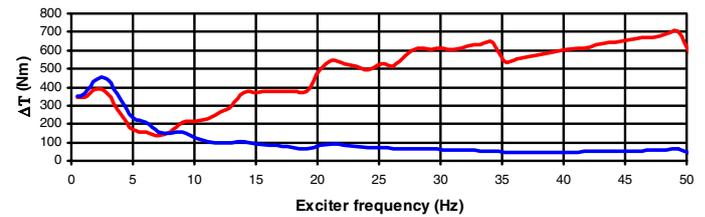
Fig. 6: Measuring values – Torque amplitudes of pump side (red) and turbine side (blue)
