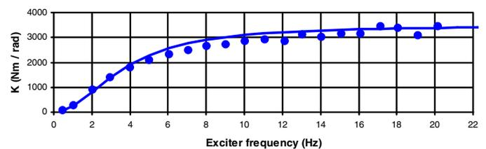
Fig. 9: Stiffness K – Measurements (dots); theory (continued)
