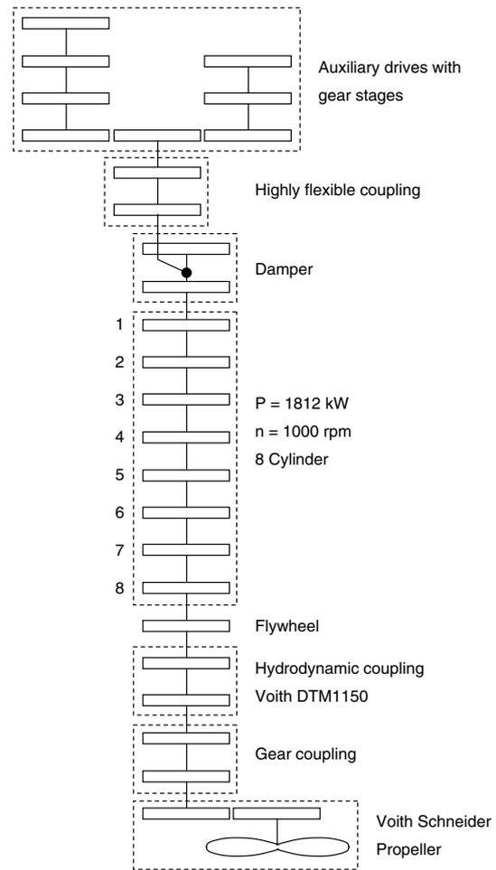
Fig. 11: Mass scheme of marine drive
