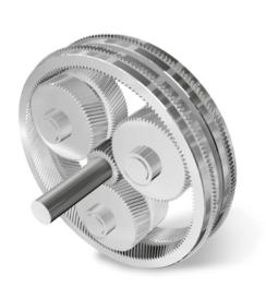
Planetary gear units need less space and weigh less in comparison to parallel shaft gear units due to the transmission of power via three or more planetary wheels.
