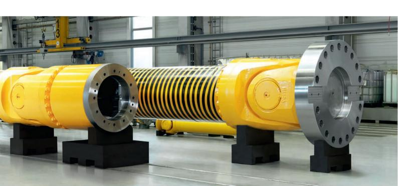
Contact with roll necks is via FlexPad metal wear plates embedded in the roll end hub body. These have an elastic compound material bonded to the plates on all surfaces contacting the REH body. The compound fully functions in an elastic range and so guarantees constantly stable positioning of the wear plates during load variations. The clearance between the roll neck and the REH remains constantly very tight during mill operations.
